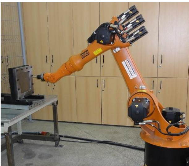
Fig. 2. Experimental layout for incremental forming
