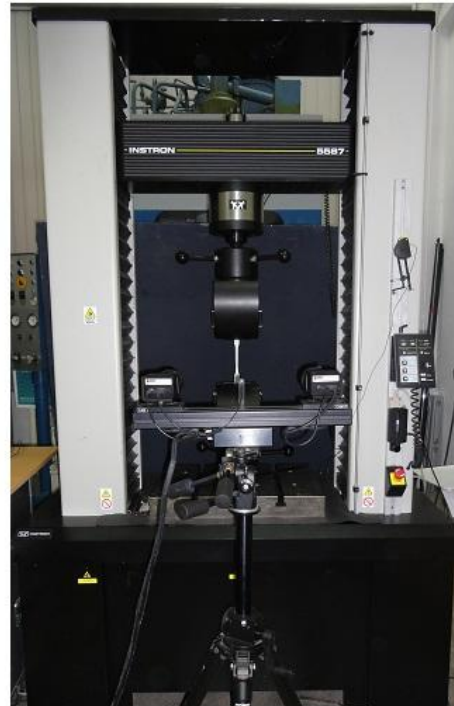
Fig. 3. Experimental layout for tensile test
