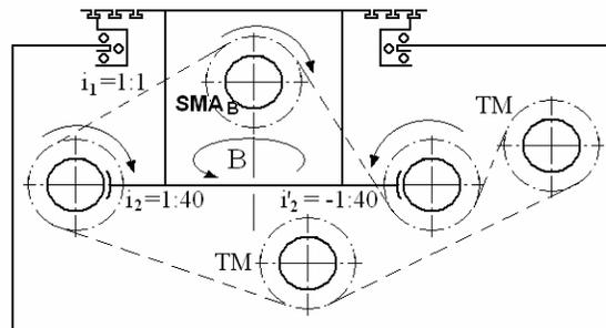
**Fig.7.Kinematic drive schematics of the worm gears at table rotation.**
