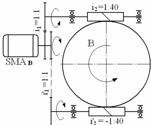
Fig.2.The kinematic schematic diagram for the spur gears and the toothed transmission belt.
