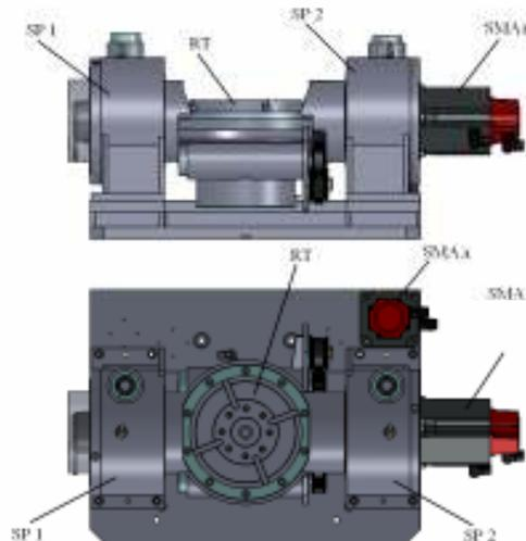
Fig.5.Rotary-tilting table RTT-5 with 250 mm shelf diameter
