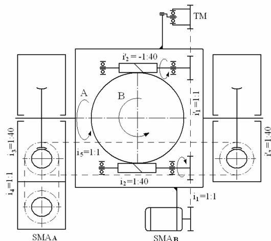
Fig.1.Kinematic schematic diagram of the rotary-tilting table family RTT-5
