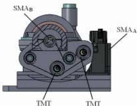
**Fig.9. The synchronous transmission solution at the continuous rotation axis.**
