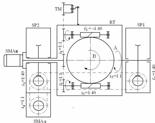
Fig.4.Kinematic schematic diagram of the rotary-tilting table RTT-5 with 250 mm shelf diameter
