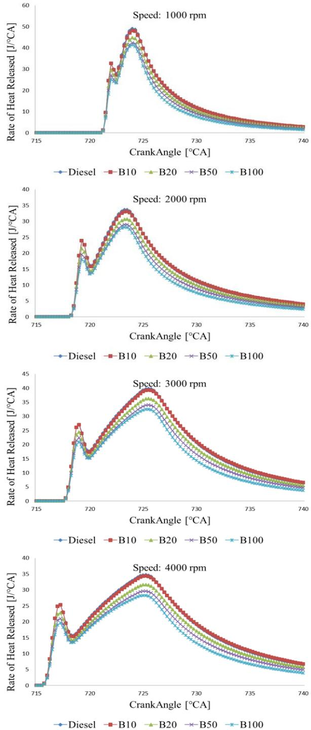
Fig. 3. Simulation results for the rate of heat released ROHR.
