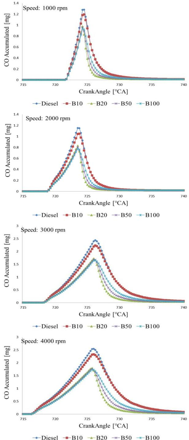
Fig. 5. Emissions of CO in the simulations with biodiesel.
