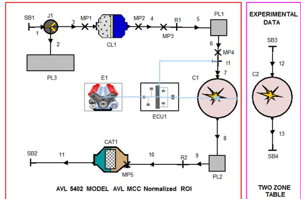
Fig. 1. The simulation model for the engine AVL 5402 in Boost with two combustion models.
