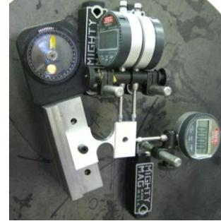
Fig. 6. Experimental setup for measuring the planar compliances
