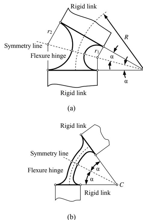
Fig. 2. Circular-axis flexure hinges: (a) Right circular; (b) Right circularly corner-filleted (radius of median circle is  $R$ )
