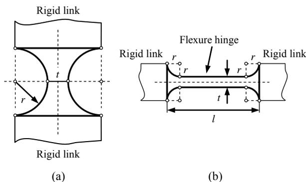
Fig. 1. Two common straight-axis flexure hinges: (a) Right circular; (b) Right circularly corner-filleted
