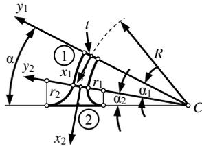
Fig. 7. Half of the circular-axis symmetric right circularly corner-tilted flexure hinge with defining geometry
