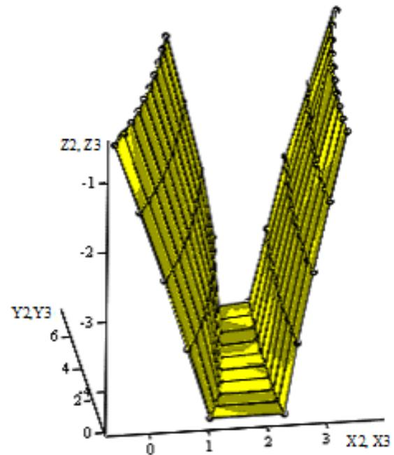
Fig. 4. The topography of the gap between the teeth done with the experimental knives
