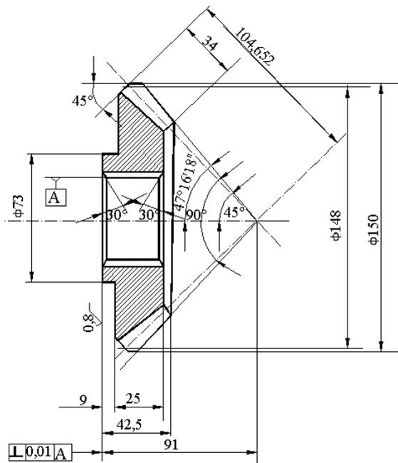
Fig. 2. The toothed wheel used for testing
