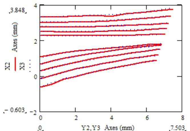
Fig. 5. A comparison of the gaps between the teeth's topography made with the experimental knives after the second and third sharpening
