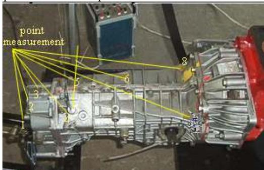
Figure 2 Gearbox Sensor Configurations
