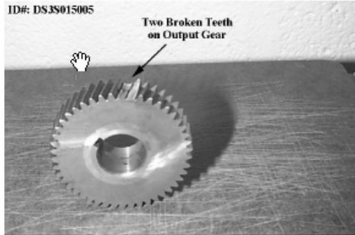
Figure 1. Two Adjacent Gear Teeth Fractures
