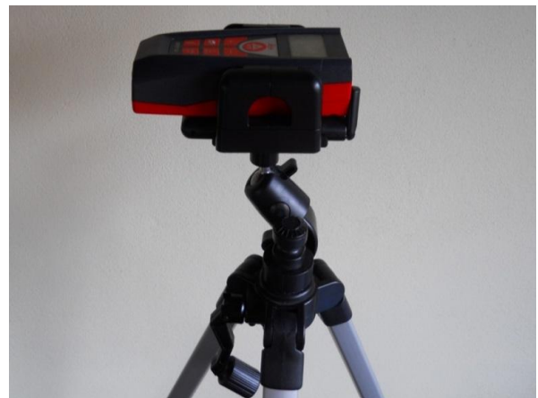
Fig. 2. Measuring device with the laser telemeter.
