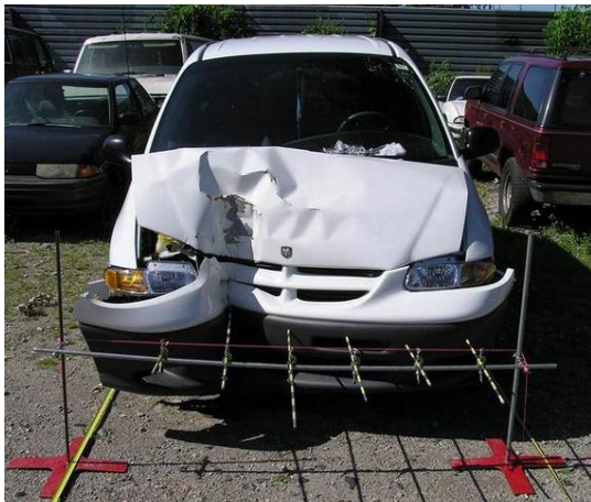
Fig. 1. Measuring the deformed profile with the profilometer
