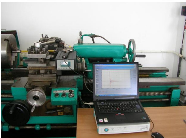
Fig. 7. Measurement system for determining the dynamic characteristics of the fiberglass reinforced epoxy resin rod
