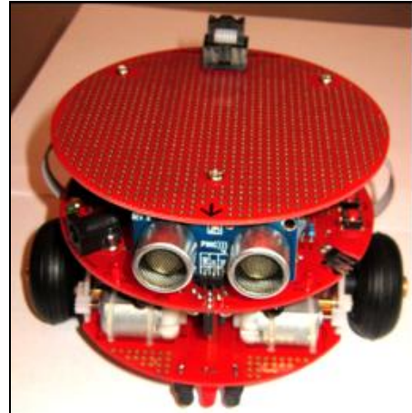
Fig. 7. Pro-Bot 128 mobile robot, equipped with a Parallax ultrasonic sensor
