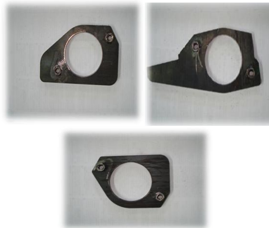
Fig. 8. The look of the welded parts (rings)
