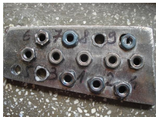
Fig. 6. Experimental setting of the welding technology - M8 nut
