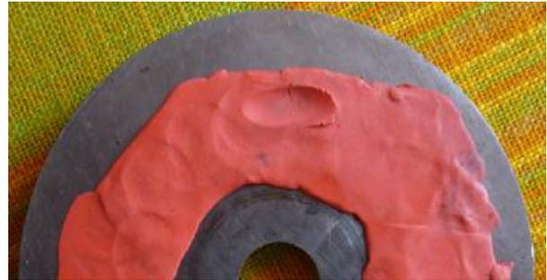
Fig. 3. For a soft material the plastic indentation does not present a plane of symmetry
