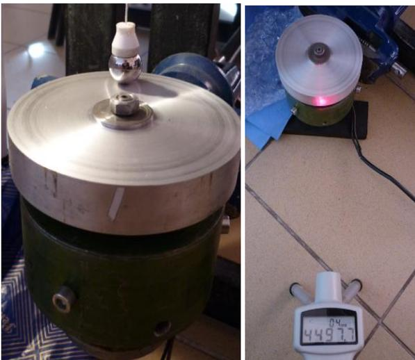
Fig. 1. Experimental device: disc mounted on motor's shaft (left) and angular velocity measurement (right)
