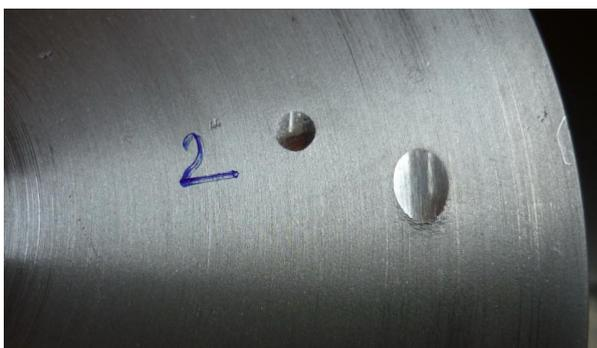
Fig. 2. Plastic imprints resulted from impact with two different size balls
