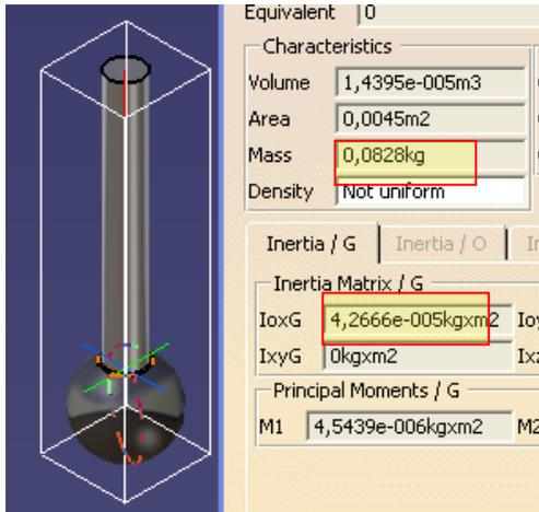
Fig. 4. Estimation of the moment of inertia about the centre of mass  $J_z$  using CAD software
