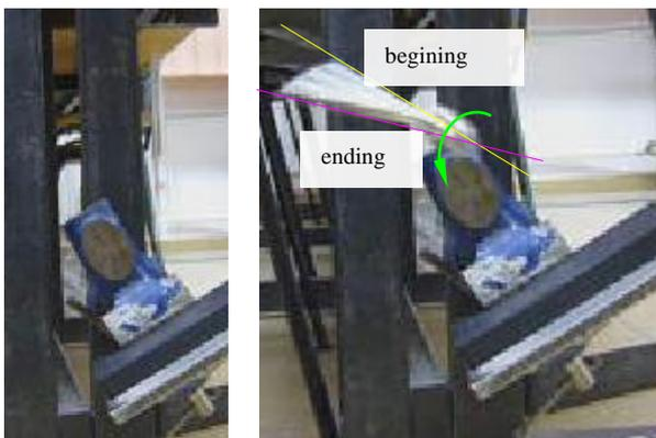
Fig. 5. The ball with the long rod before and after impact
