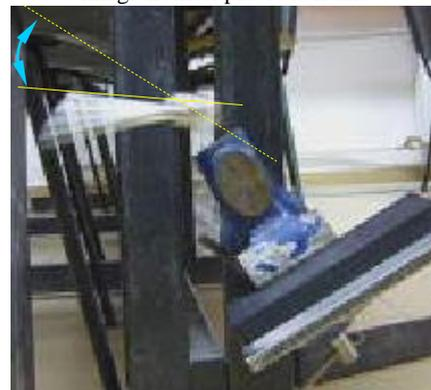
Fig. 7. Estimation of rotation angle between two successive image frames: present frame
