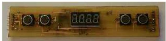
Fig. 1.12. Final timer board with electronic components
