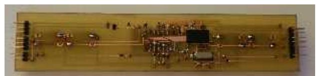
Fig. 1.13. Final timer board with electronic components
