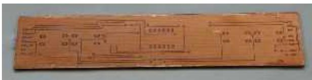
Fig. 1.9. Circuit diagram transferred on the plate - side two
