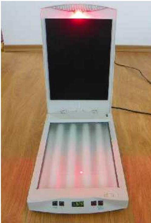
Fig. 1.14. Scanner housing converted to ultraviolet light exposure system use for PCB-s technology
