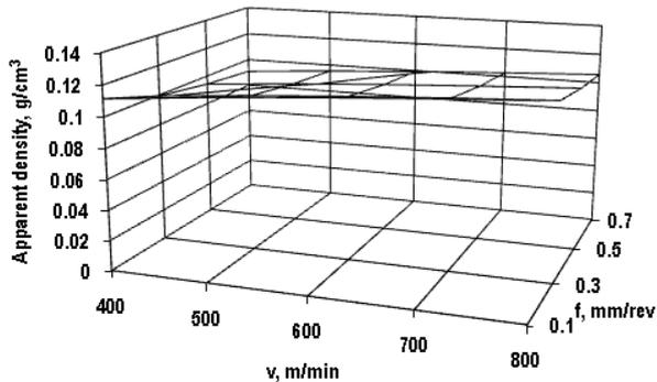
Fig. 6. Influence of the milling speed  $v$  and feed rate  $f$  on the chips apparent density  $\rho_a$  ( $HRC=55$ ,  $a_p=0.5$  mm).
