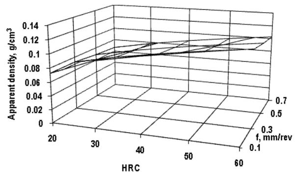
Fig. 4. Influence of the test piece material hardness  $HRC$  and feed rate  $f$  on the chips apparent density  $\rho_a$  ( $v=600$  m/min,  $a_p=0.5$  mm).
