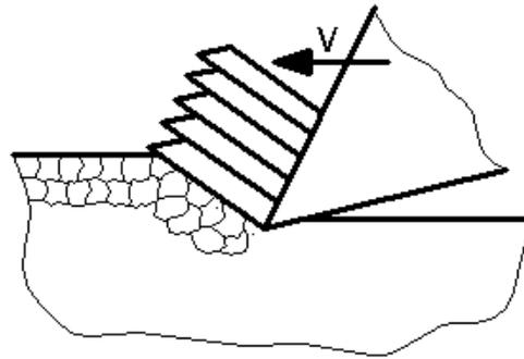
Fig. 1. Chip generation during the process of high speed milling of hard materials.
