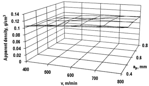
Fig. 7. Influence of the milling speed  $v$  and depth of cut  $a_p$  on the chips apparent density  $\rho_a$  ( $HRC=55$ ,  $f=0.3$  mm/rev).
