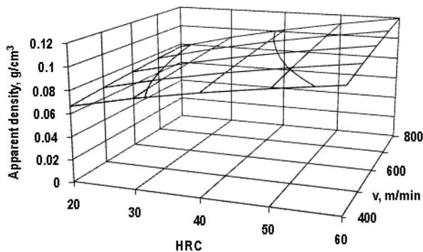
Fig. 3. Influence exerted by the test piece material hardness  $HRC$  and milling speed  $v$  on the chips apparent density  $\rho_a$  ( $f=0.3$  mm/rev,  $a_p=0.5$  mm).
