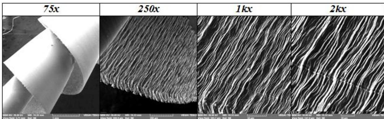
Fig. 2. Aspect of the chips obtained by face milling on test pieces of tools steel X210Cr12 ( $HRC=59$  HRC,  $v=408.4$  m/min,  $f=0.63$  mm/rot,  $a_p=0.5$  mm; images obtained by means of the scanning electron microscope Vega II Tescan LSH).
