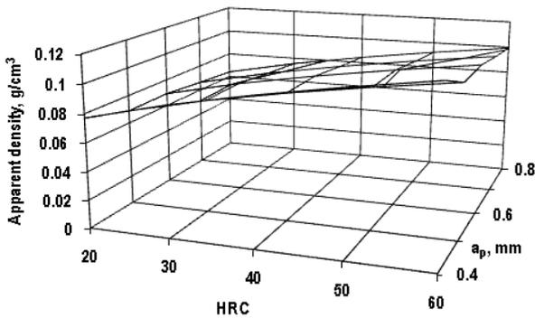
Fig. 5. Influence of the test piece material hardness  $HRC$  and depth of cut  $a_p$  on the chips apparent density  $\rho_a$  ( $v=600$  m/min,  $f=0.3$  mm/rev).
