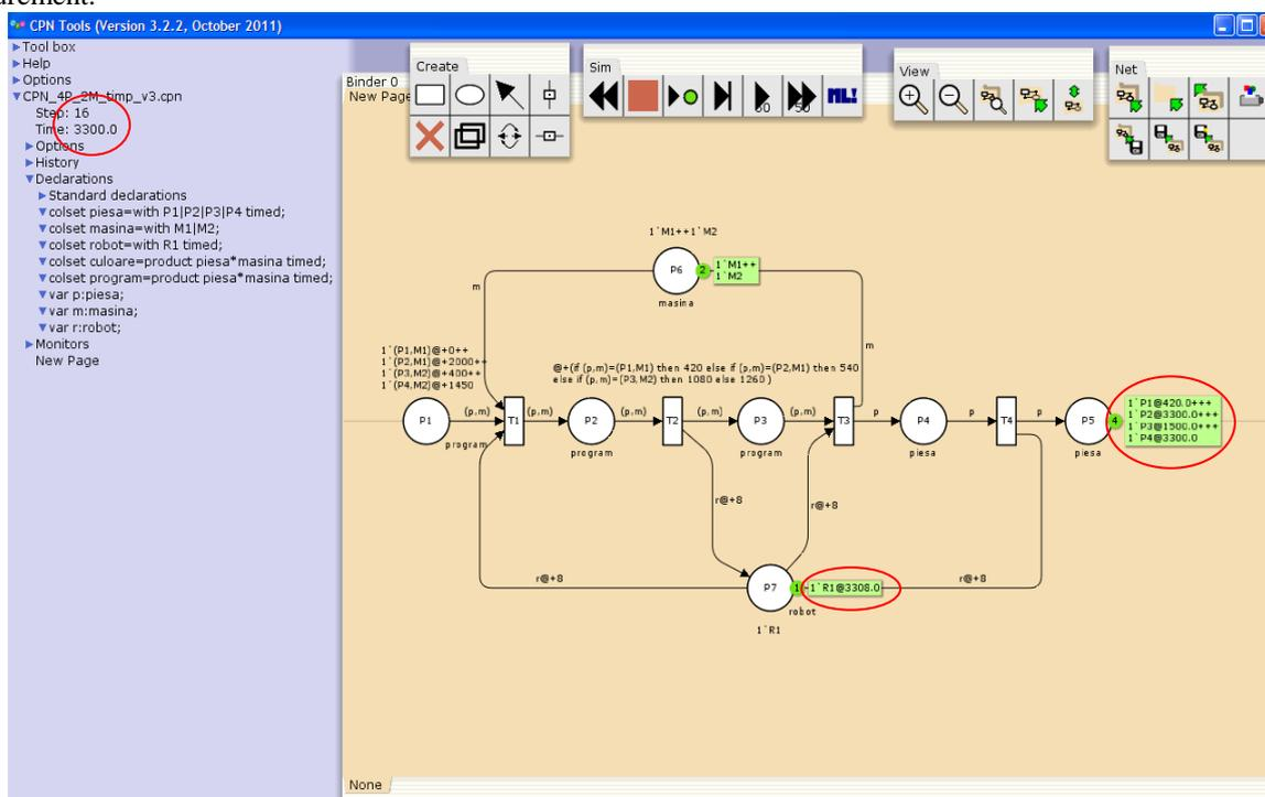
Fig. 5. Timed coloured Petri Net model, after simulation
