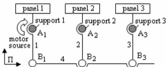
Fig. 1. The structural model of the tracking mechanism for the daily motion.
