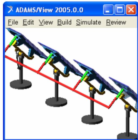
Fig. 2. The virtual prototype of the PV string with dual-axis tracking system.
