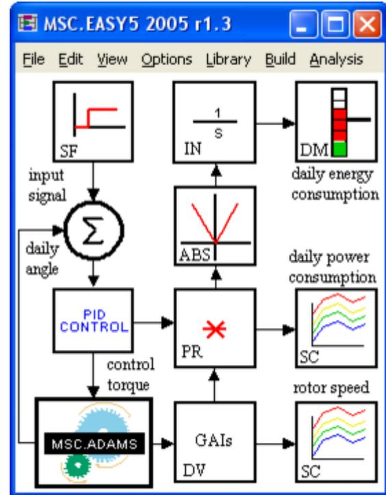
Fig. 4. The control system block diagram for the daily motion.
