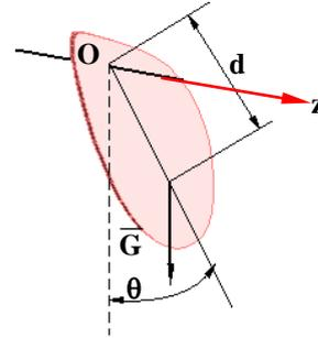
Fig. 1. Physical pendulum
