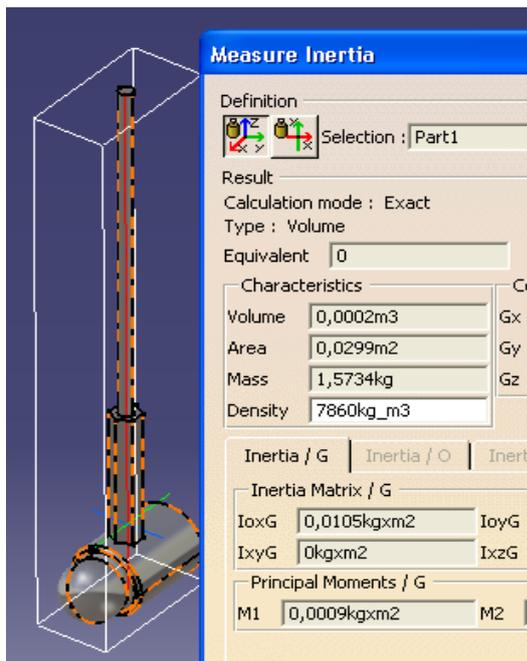
Fig. 5. The axial moment of inertia for a hammer pendulum obtained by CAD model
