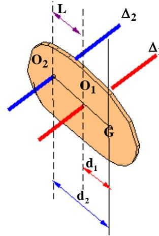
Fig. 2. Physical pendulum and the two oscillation axes
