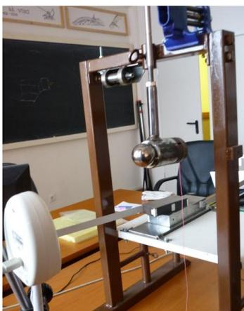
Fig. 6. The axial moment of inertia for a hammer pendulum obtained using the present method
