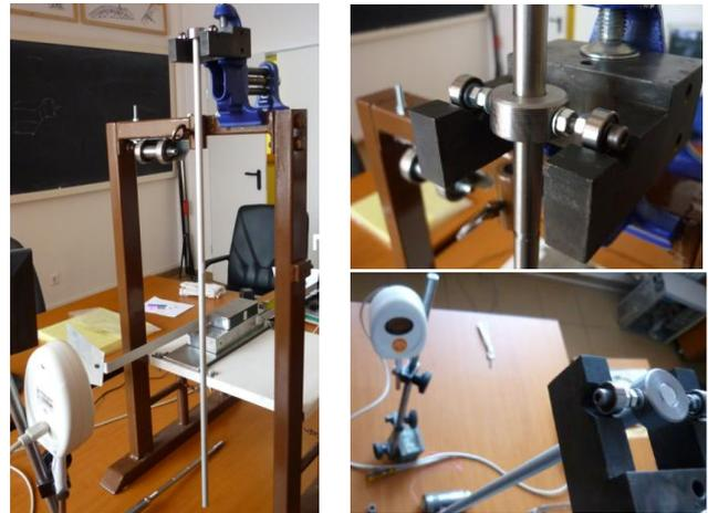
Fig. 3. System used for finding the period of oscillation
