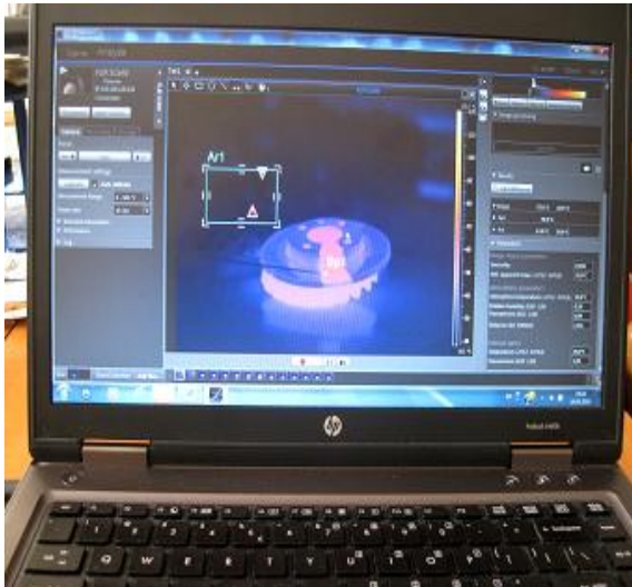
Fig. 1. The picture of the disc brake viewed with thermovision camera
