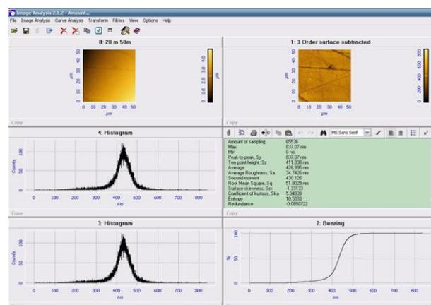
Fig. 5. Specific parameters obtained using AFM surface quality in the center bounded by the red marker (before the start).
