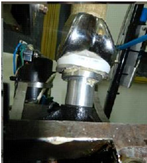
Fig. 7. Mounting of the LCS Mobile-Bearing Total Knee System on the stand (detail).
