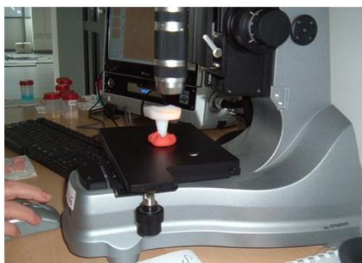
Fig. 3. Visual inspection of the articular surfaces of the UHMWPE component using KEYENCE VHX-600E.
