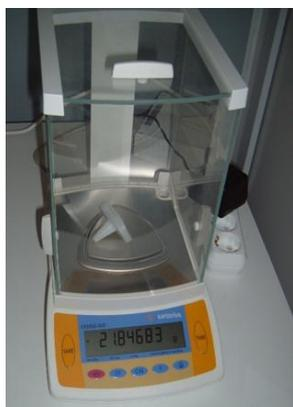
Fig. 2. Weighing of UHMWPE component.
