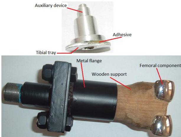
Fig. 6. Auxiliary devices used to fix the LCS Mobile-Bearing Total Knee System on the experimental stand
