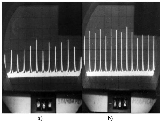
Fig. 1. The cyclic dispersion: a) for series engine; b) gasoline-hydrogen engine
