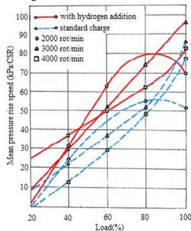
Fig. 6 The variation of the pressure rise speed
