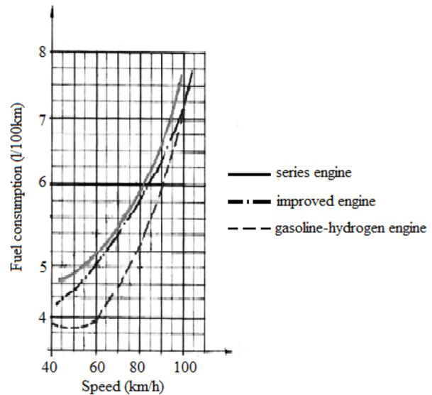
Fig. 8. Fuel consumption for three different engines
