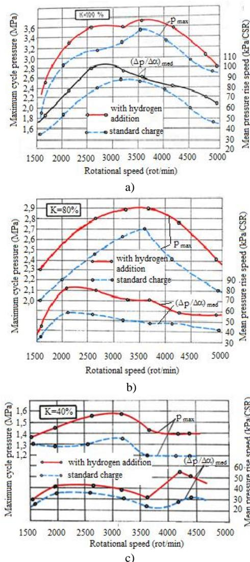
Fig. 4 The maximum engine cycle pressure for: a)  $K=100\%$ ; b)  $K=80\%$ ; c)  $K=40\%$
