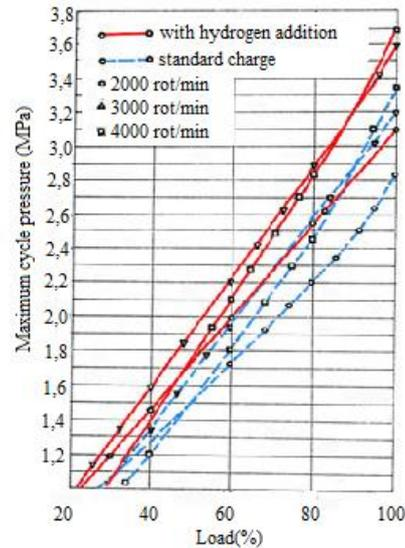
Fig. 5 The maximum engine cycle pressure for different rotational speeds
