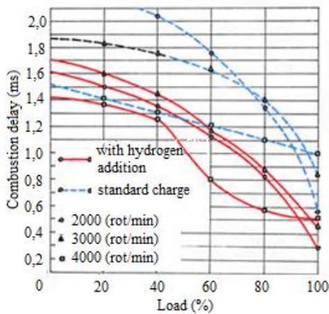
Fig. 3. Combustion delay at three different rotational speeds
