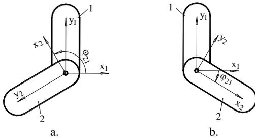
Fig. 5. Joint relative rotation angle measurement
