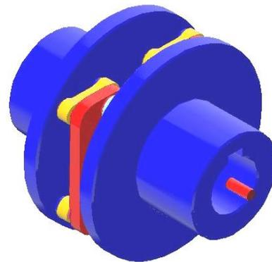
Fig. 3. Coupling virtual model
