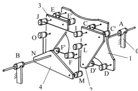
Fig. 1. Transversal mobile coupling structural scheme and the associated mechanism
