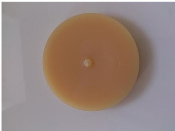
Fig. 2. The PA66 polyamide rough disk
