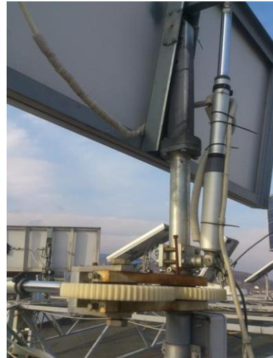
Fig. 1. Solar tracking system with polyamide gear
