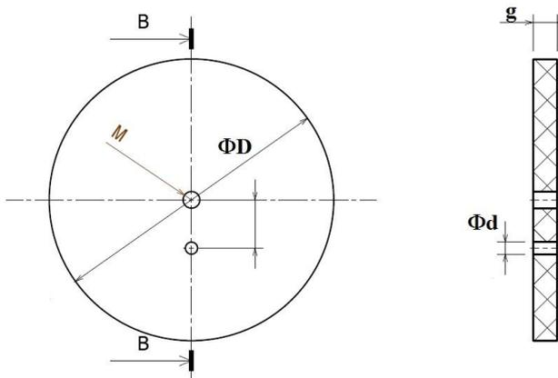
Fig. 3. The PA66 disks draft drawing
