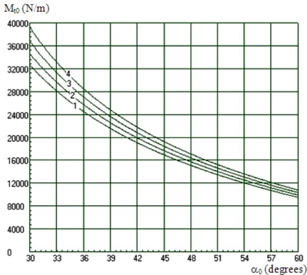
Fig. 10. Variation of torque transmitted by the clutch for different friction coefficient values  $\mu_0$  ( $D_0=150$  (mm),  $d_b=12$  (mm),  $\alpha_1=30^\circ$ ,  $r=3$  (mm),  $c=43$  (N/mm),  $h_1=1.5$  (mm),  $\mu_1=\mu_2=0.08$ ).
