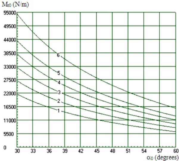
Fig. 7. Variation of torque transmitted by the clutch for different values of the diameter of balls arrangement ( $d_b=12$  (mm),  $\alpha_1=30^\circ$ ,  $r=3$  (mm),  $\delta_1=2$  (mm),  $c=43$  (N/mm),  $h_1=1.5$  (mm),  $\mu_0=0.06$ ,  $\mu_1=\mu_2=0.08$ ).
