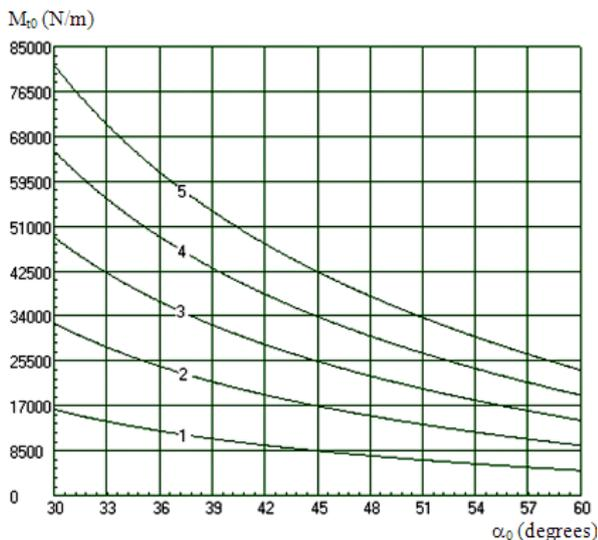
Fig. 8. Variation of torque transmitted by the clutch for different values of arc compression during assembly ( $D_0=150$  (mm),  $d_b=12$  (mm),  $\alpha_1=30^\circ$ ,  $r=3$  (mm),  $c=43$  (N/mm),  $h_1=1.5$  (mm),  $\mu_0=0.06$ ,  $\mu_1=\mu_2=0.08$ ).
