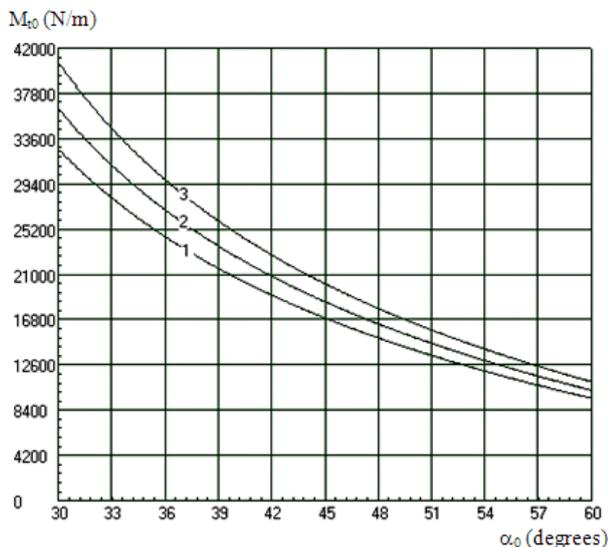
Fig. 11. Variation of torque transmitted by the clutch depending on the friction coefficients  $\mu_{01}$  and  $\mu_{02}$  ( $D_0=150$  (mm),  $d_b=12$  (mm),  $\alpha_1=30^\circ$ ,  $r=3$  (mm),  $c=43$  (N/mm),  $h_1=1.5$  (mm),  $\mu_0=0.06$ ).
