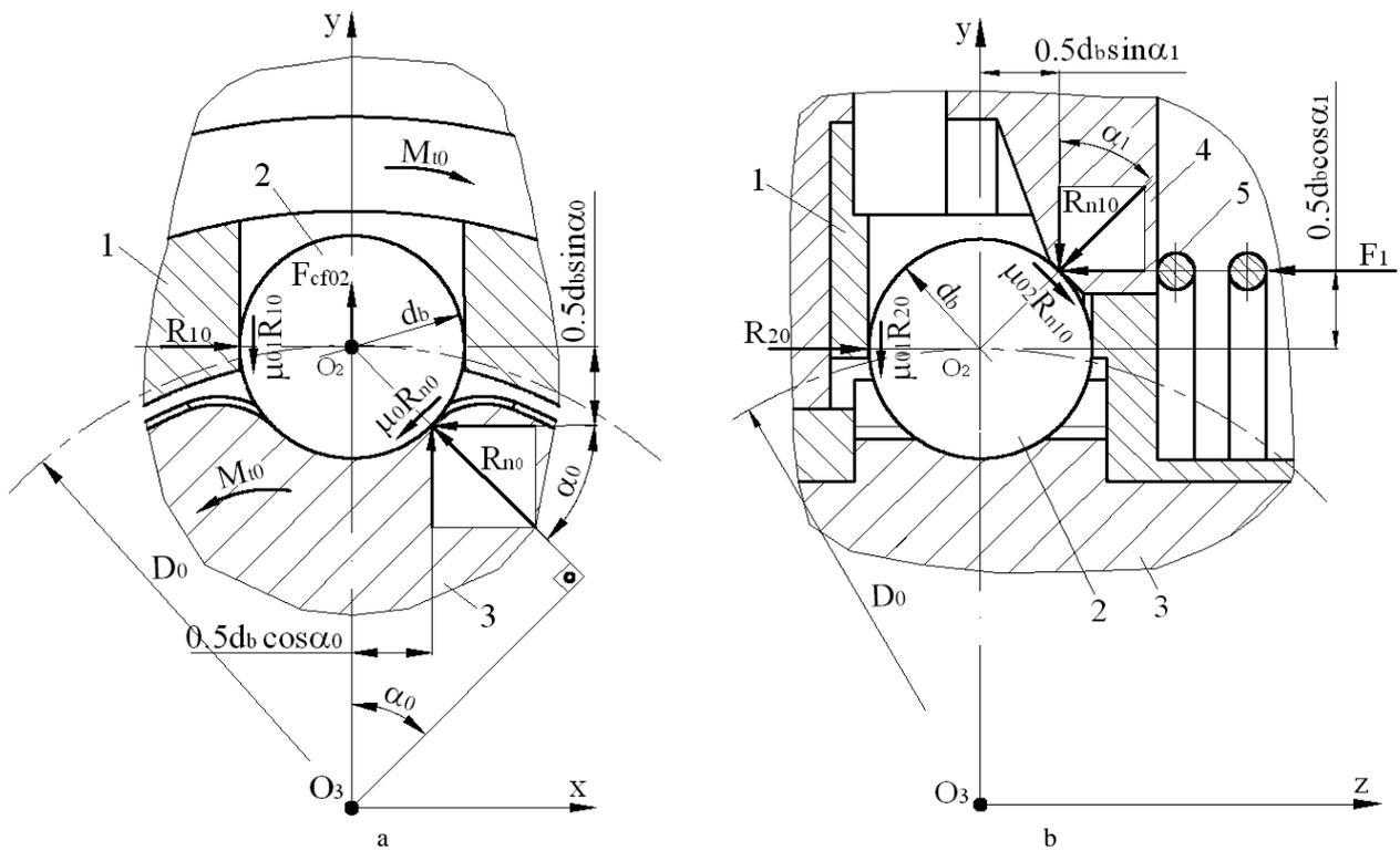
Fig. 3. Clutch model for the complete engaged working. a – frontal section; b – longitudinal section
