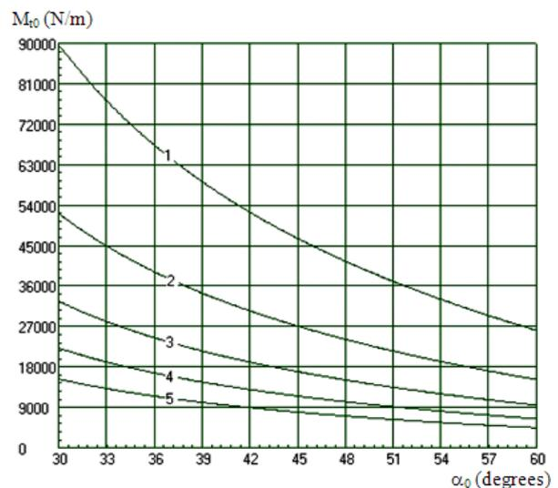
Fig. 9. Variation of torque transmitted by the clutch considering different values of the angle of the first inclined part of the pressure plate ( $D_0=150$  (mm),  $d_b=12$  (mm),  $r=3$  (mm),  $h_1=1.5$  (mm),  $\mu_0=0.06$ ,  $\mu_1=\mu_2=0.08$ ).
