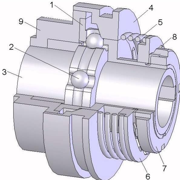
Fig. 1. Complete engaged clutch
