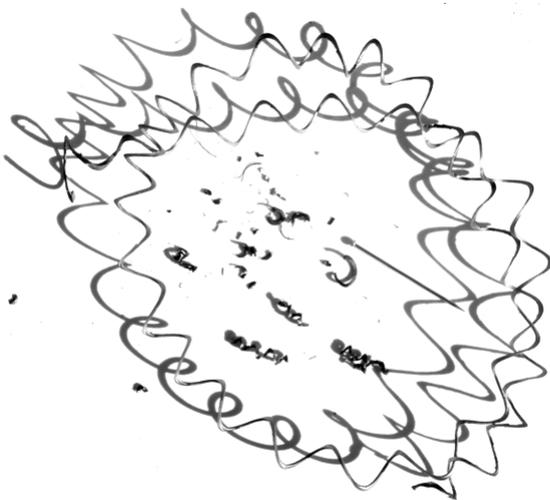
Fig. 7. The aspect of resulted chips after turning the sample 5 with feed  $f = 0.5\text{mm/rot}$
