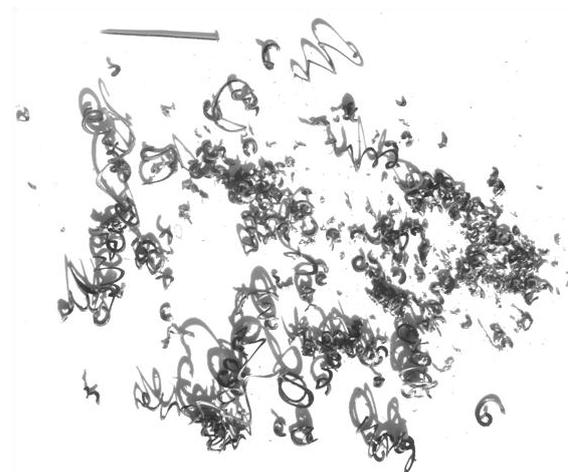
Fig. 5. The aspect of resulted chips after turning the sample 3 with feed  $f = 0.302 \text{ mm/rot}$
