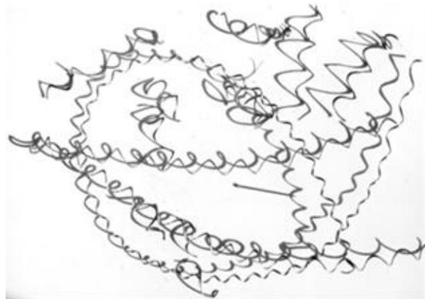
Fig. 4. The aspect of resulted chips after turning the sample 2 with feed  $f = 0.209 \text{ mm/rot}$
