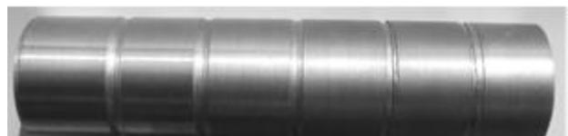
Fig. 1. The shaft with diameter of  $\Phi 34$  mm machined by turning
