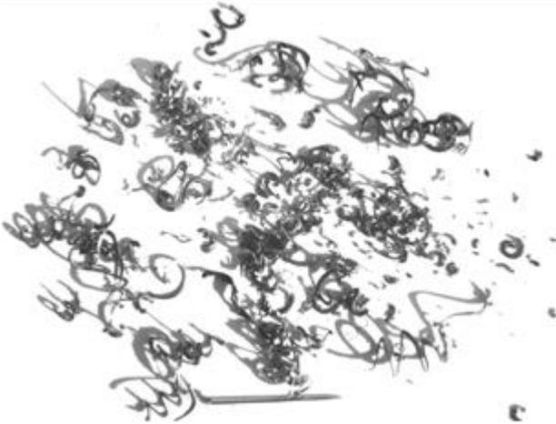
Fig. 6. The aspect of resulted chips after turning the sample 4 with feed  $f = 0.416\text{mm/rot}$
