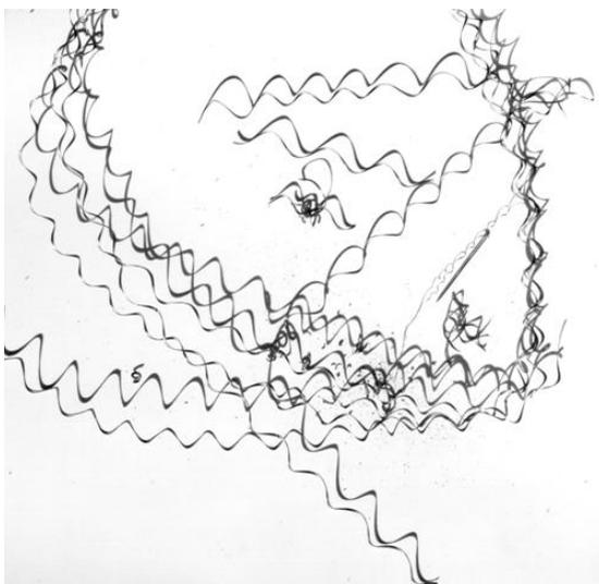
Fig. 3. The aspect of resulted chips after sample 1 turning with feed  $f = 0.096 \text{ mm/rot}$
