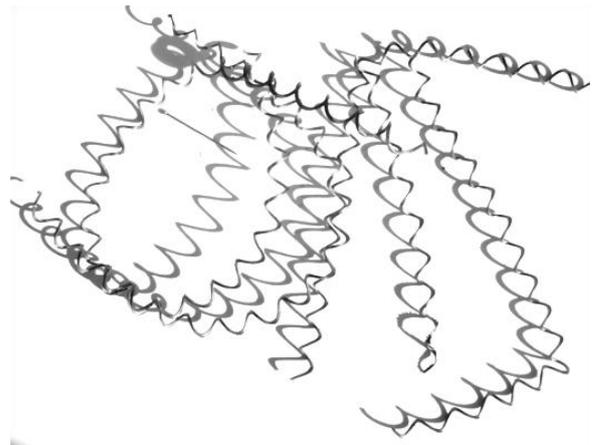
Fig. 8. The aspect of resulted chips after turning the sample 6 with feed  $f = 0.584\text{ mm/rot}$
