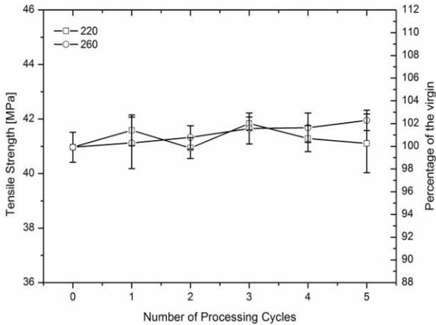
Fig. 1. Tensile strength for the reprocessed ABS.
