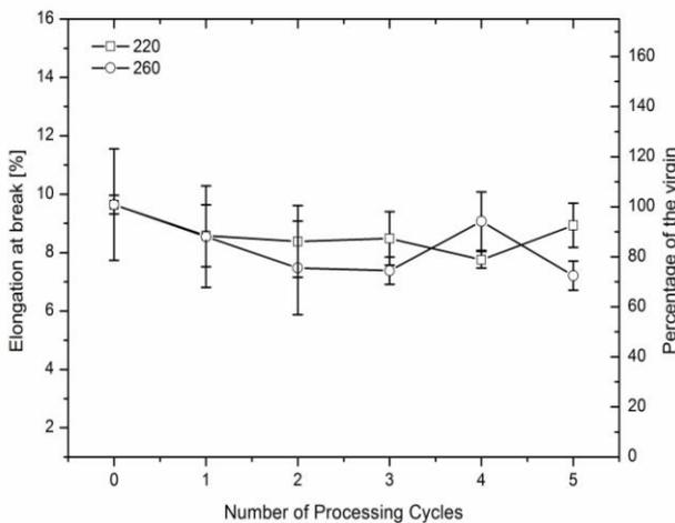
Fig. 2. Elongation at break for the reprocessed ABS.
