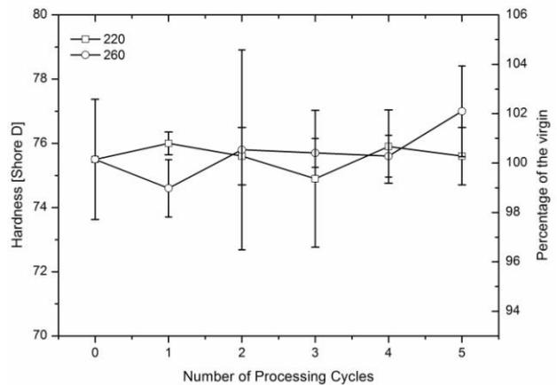
Fig. 4. Hardness for the reprocessed ABS.
