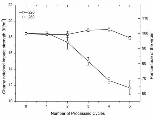
Fig. 3. Impact strength for the reprocessed ABS.
