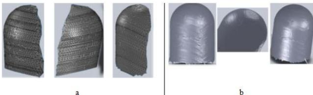
Fig. 5 Showing sensing methods of welding tip geometry - version No.4
