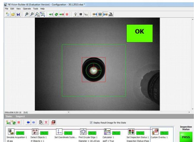
Fig. 6 Showing the working environment of the program Vision Builder with successful image processing
