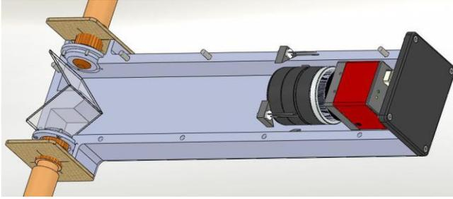
**Figure 7** showing a 3D model for recording and evaluation of the surface of both tips of welding heads
