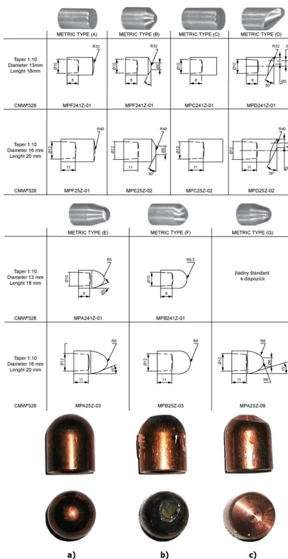
Fig. 1 Welding electrodes [6] tips comparison: a) new, b) worn, c) restored
