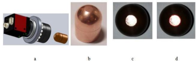
Fig.3. Showing sensing methods of welding tip geometry - version No.2
