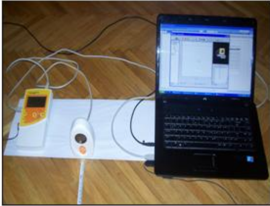
Fig. 5. Ultrasonic sensor attached to data acquisition system and notepad
