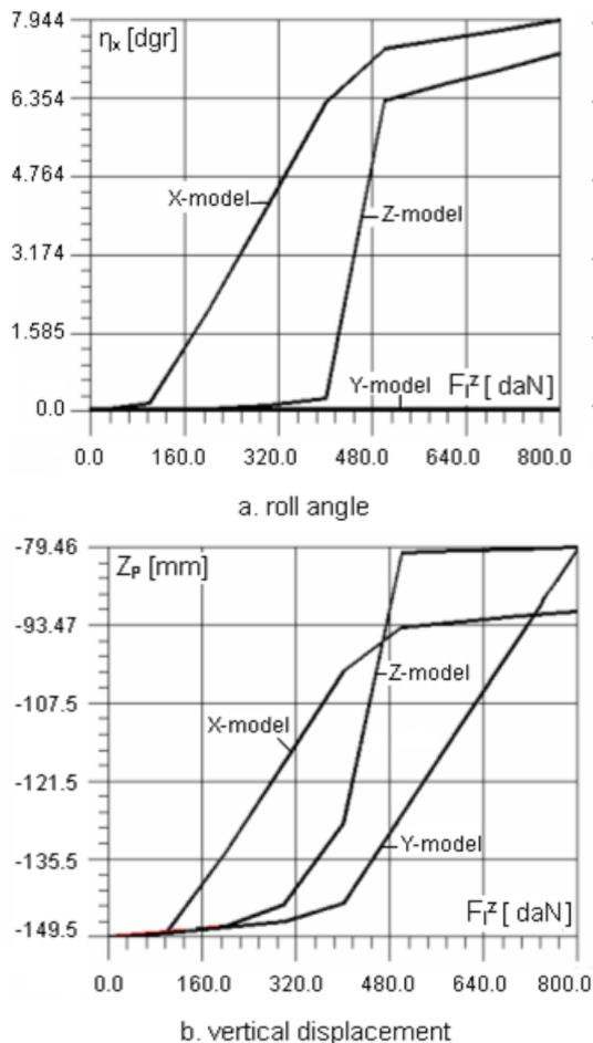
Fig. 5. The results of the static analysis for the guiding linkages with 4-DOF joint models.
