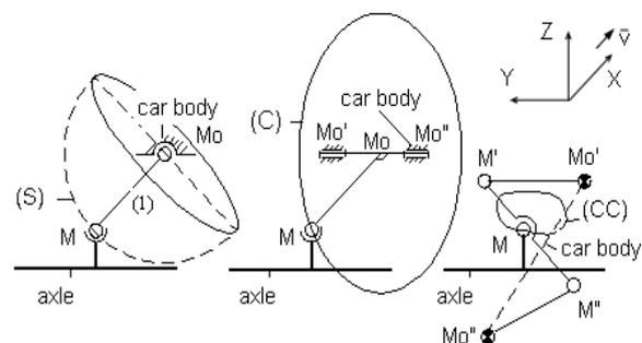
Fig. 1. The basic types of guidance for the rear axle of the vehicles [3].
