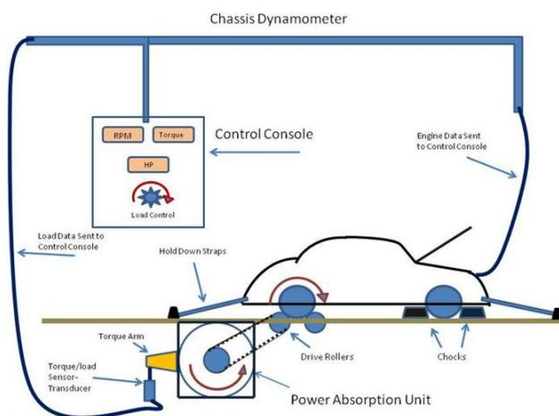
Fig. 1. Chassis dynamometer setup [15]
