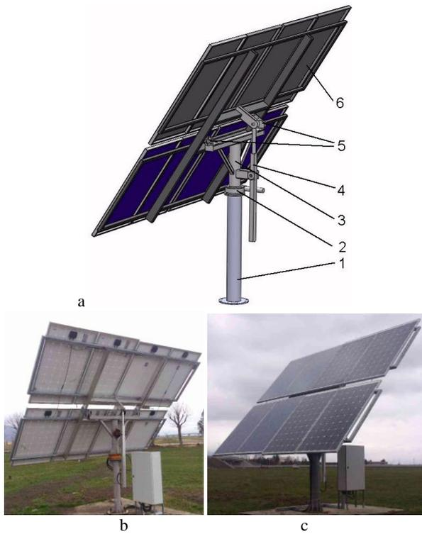
Fig. 4. Components of the azimuthal tracker driven by one slew drive and one linear actuator.
