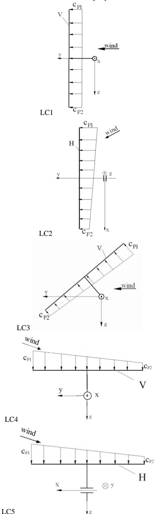
Fig. 3. Wind load cases for PV platforms calculus.
