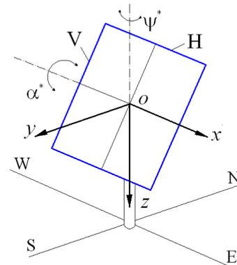
Fig. 1. General diagram of an azimuthal solar tracking system.
