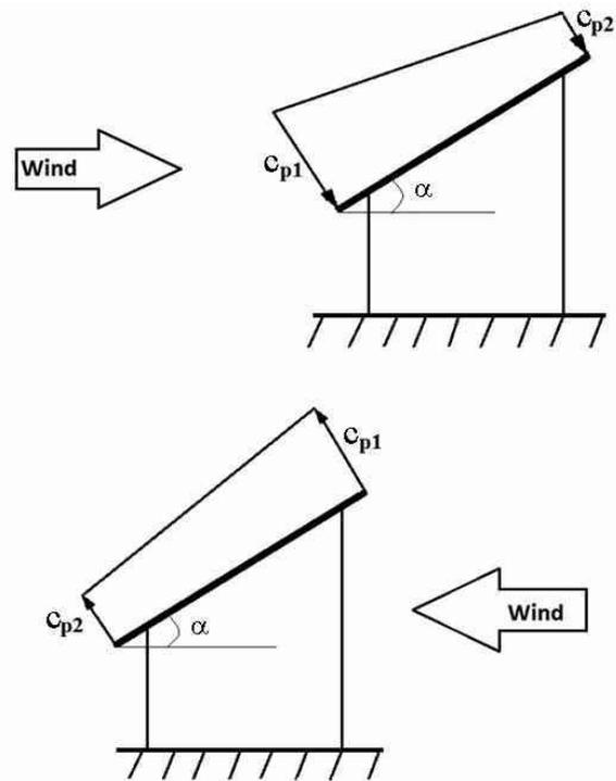
Fig. 2. Pressure coefficients and distribution diagram on PV platforms.
