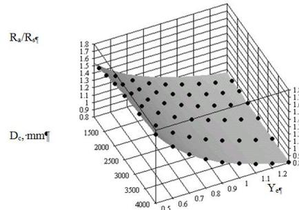
Fig. 3. The influence of quality level of the tool exploitation  $Q_l$  on change of the actual flow  $R_a$  compared with standard  $R_s$  for machine tools of different  $D_c$  sizes
