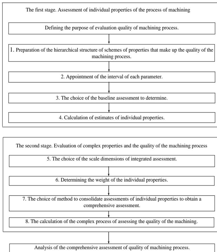
Fig. 2. - An algorithm of complex evaluation of the quality of machining processes
