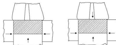
Fig. 1. Meaning heat flow of the heating cavity of the mould
