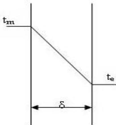
Fig. 2. The heat lost by conductivity
