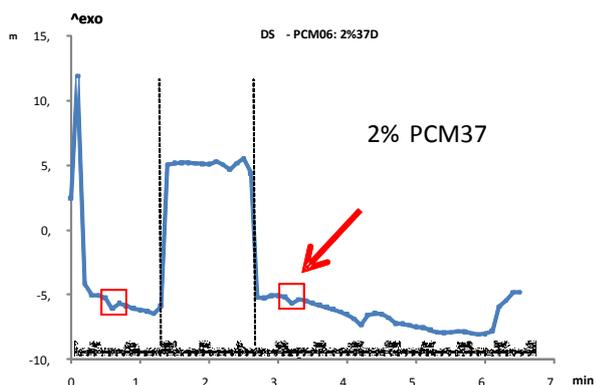
Fig. 3. DSC calorimetric curve generated by the mixture of SEBS PCM06, subjected to a heating-cooling cycle overheating.
