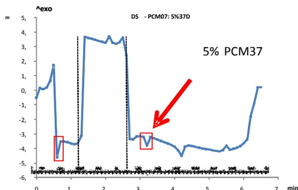
Fig. 4. DSC calorimetric curve generated by the mixture of SEBS PCM07, subjected to a heating-cooling cycle overheating.
