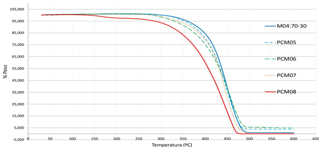
Fig. 6. Thermogravimetric comparative curves of SEBS blends (%weight vs temperature).
