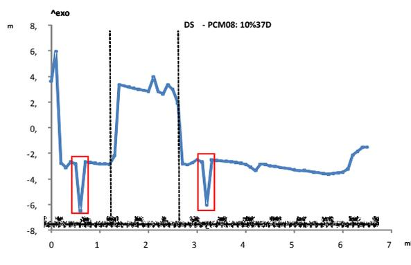
Fig. 5. DSC calorimetric curve generated by the mixture of SEBS PCM08, subjected to a heating-cooling cycle overheating.
