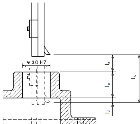
Fig. 2. 2D modeling of the  $l_c$  working stroke length determination
