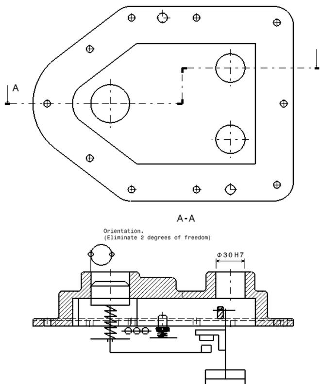
Fig. 3. 2D modeling of the half-shell landmark's guidance system in the device
