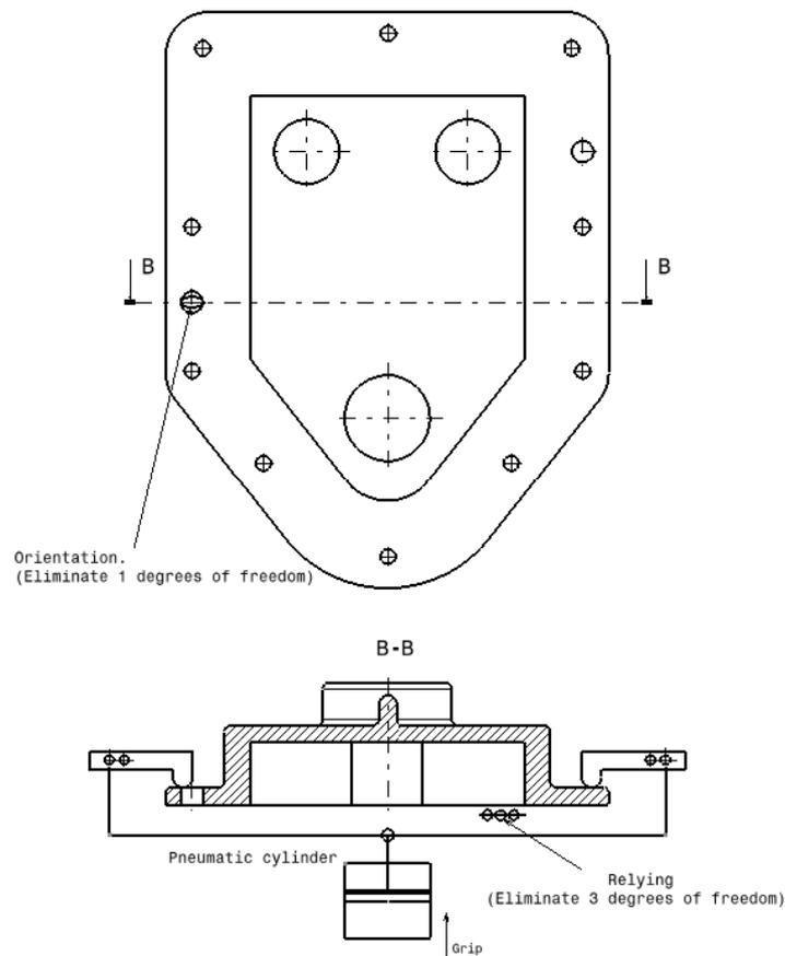
Fig. 4. 2D modeling of the pneumatically actuated centering and fastening system with levers
