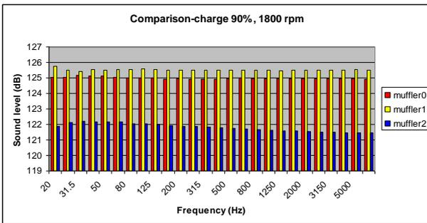
Fig. 10. Sound level comparison - load 90%, 1800 rpm.
