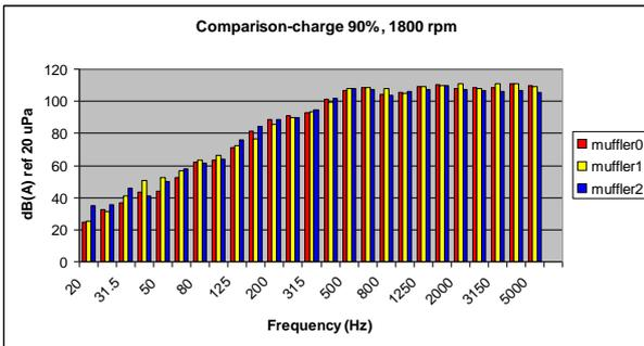
Fig. 9. Third octave comparison - load 90%, 1800 rpm
