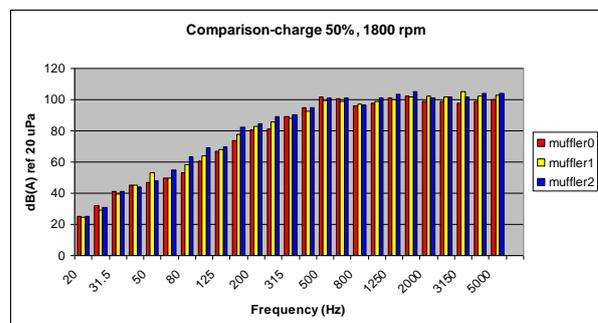
Fig. 7. Third octave comparison - load 50%, 1800 rpm
