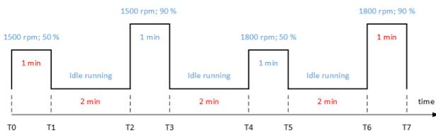
Fig. 4. Measuring cycle of the engine
