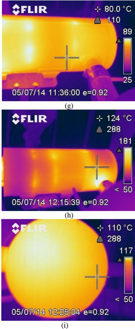
Fig. 11. Thermographic images with temperature distribution and high temperature areas on the exterior muffler surface
