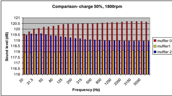
Fig. 8. Sound level comparison - load 50%, 1800 rpm
