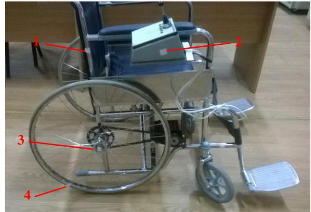
Fig.16. Positioning of reflective markers on the wheelchair.
