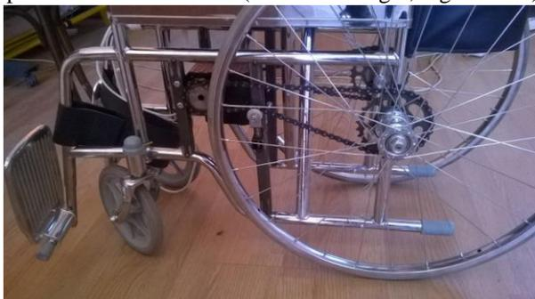
Fig. 2.Aspect of the wheelchair chain transmissions.
