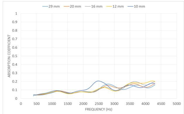
Fig.4. Shows the influence of the thickness in the the sound absorption coefficient in EVA samples of density of 300 kg/m3.
