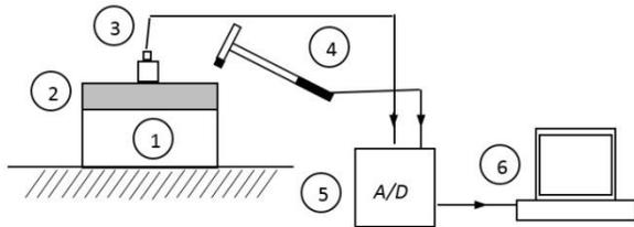
Fig. 2. Apparatus used to measure the dynamic stiffness, 1) is the test specimen; 2) is the upper steel plate; 3) the accelerometer (PCB 352C42); 4) the impact hammer (PCB 086C01); 5) the data acquisition card (NI-9233) and 6) the PC.
