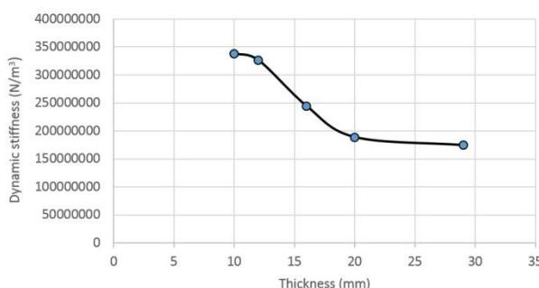
Fig.6. Influence of the thickness in the dynamic stiffness in EVA samples of density of 300 kg/m<sup>3</sup>.
