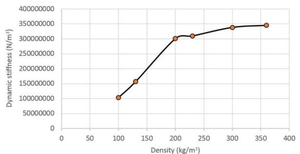
Fig.5. Influence of the density in the dynamic stiffness in EVA samples of thickness 10 mm.
