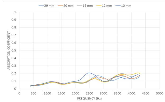
Fig.4. Shows the influence of the thickness in the sound absorption coefficient in EVA samples of density of 300 kg/m³.
