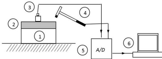
Fig. 2. Apparatus used to measure the dynamic stiffness, 1) is the test specimen; 2) is the upper steel plate; 3) the accelerometer (PCB 352C42); 4) the impact hammer (PCB 086C01); 5) the data acquisition card (NI-9233) and 6) the PC.
