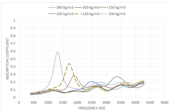
Fig.3. Shows the influence of the density in the sound absorption coefficient in EVA samples of thickness 10 mm.
