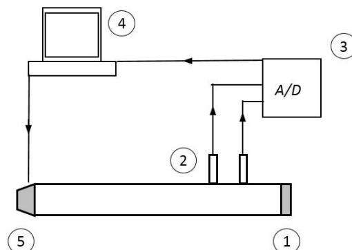
Fig. 1. Apparatus used to measure the sound absorption coefficient, where: 1) is the sample; 2) the two microphones (microphones G.R.A.S. model 40AO); 3) the data acquisition system (NI-9233); 4) the PC and 5) the sound source.
