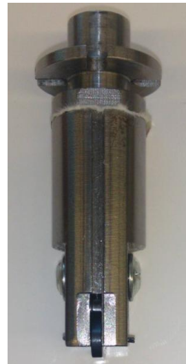
Fig. 5. The steel plate holder
