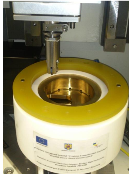
Fig. 4. The polyamide disk mounted inside the rotational device
