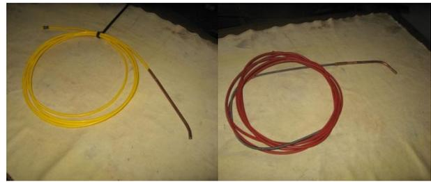
Fig. 9. The flexible guiding tube made of: raylon - left; steel – right
