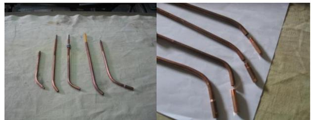
Fig. 5. Types of guiding tubes
