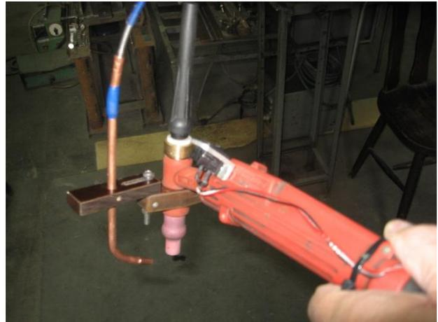
Fig. 4. The positioning and guiding head of the wire electrode
