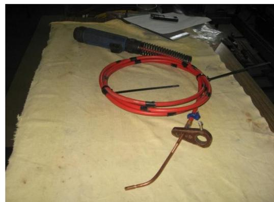
Fig. 10. The guiding tube reinforced with plastic tube
