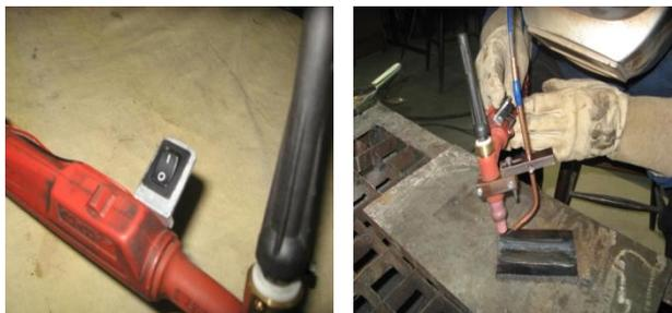
Fig. 12. Wire control switch
