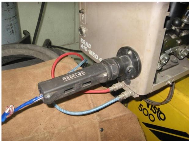
Fig. 11. Euro hitch mounted on WFD a10-med44 (ESAB)
