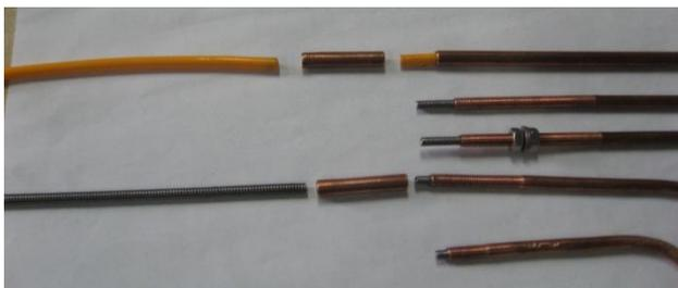
Fig. 7. Wire guiding route assembly deployed
