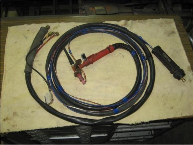
Fig. 3. Overview of WIG welding equipment
