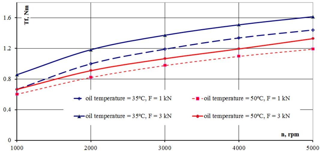
Fig. 11. Measured friction torque on bearing boxes depending on rotation, for constant tensioning force and oil temperature
