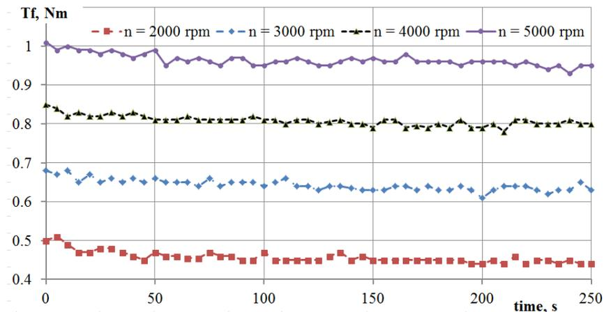
Fig. 10. Time depending friction torque for constant speed, load and oil temperature
