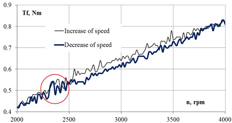
Fig. 9. Friction torque during acceleration and deceleration
