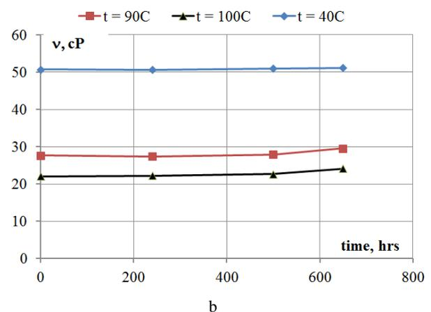
Fig. 5. Kinematic viscosity: a- versus temperature, b- versus time
