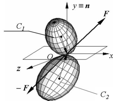
Fig. 1. Oblique collision of two bodies
