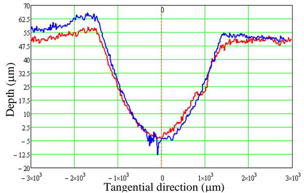
Fig. 9. Comparison between tangential profiles for inclined plane and rotating disc for  $n = 680\text{rot} / \text{min}$
