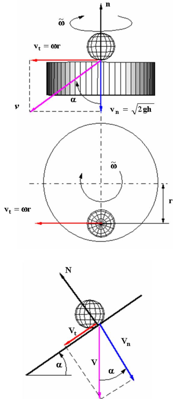
Fig. 3. Kinematical equivalence of the two collisions
