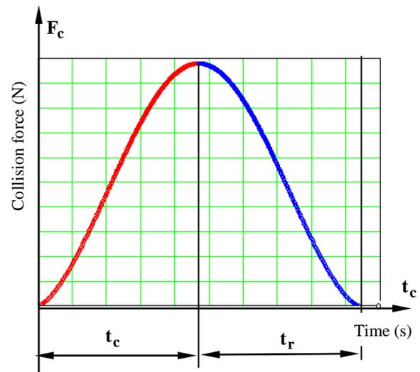
Fig. 2. Phases of collision process
