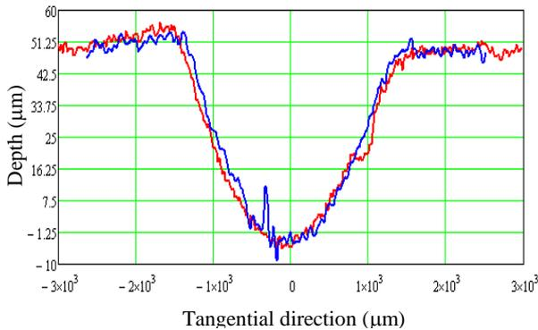
Fig. 7. Comparison between tangential profiles for  $n = 680\text{rot} / \text{min}$
