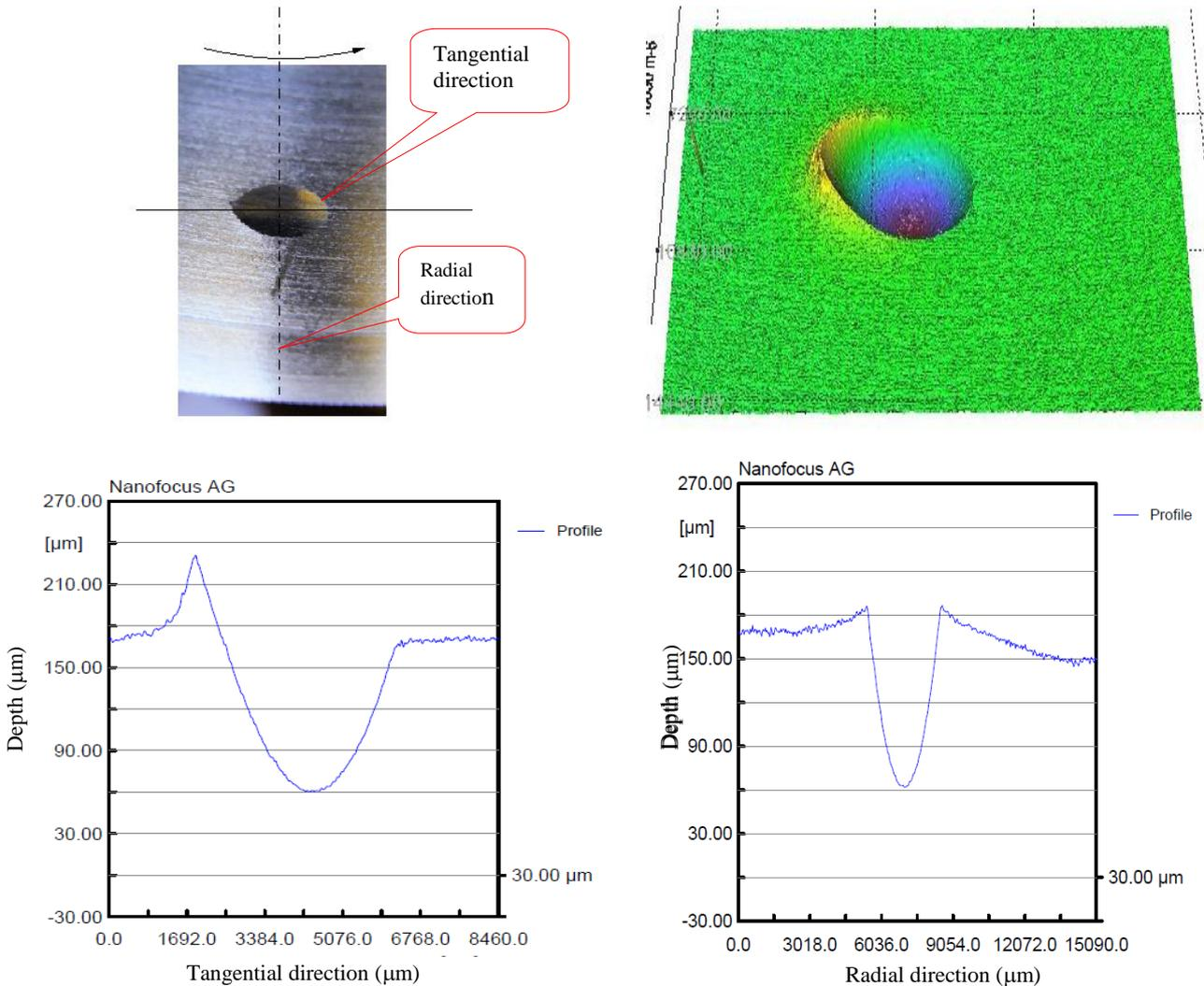
Fig. 4. Photography, 3D image, tangential and radial profiles for an indentation on an aluminum disc
