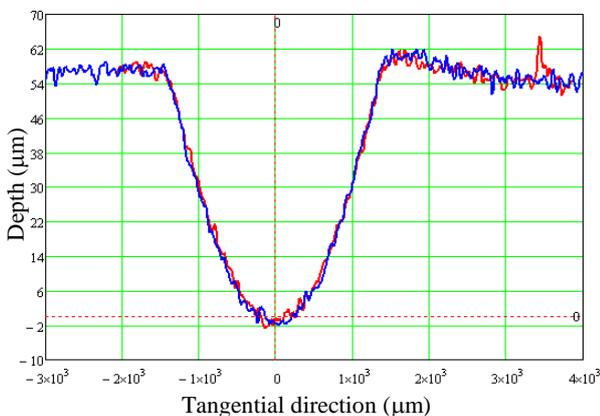
Fig. 8. Comparison between tangential profiles for inclined plane and rotating disc for  $n = 480\text{rot} / \text{min}$
