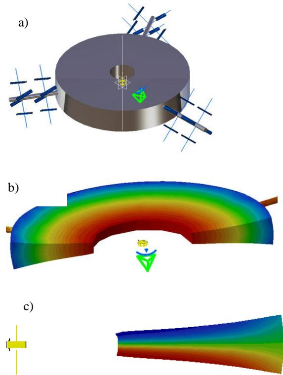
Fig. 3. FEA analysis of a disc in rotation: a) imposed constraints; b) stress field; c) deformed shape
