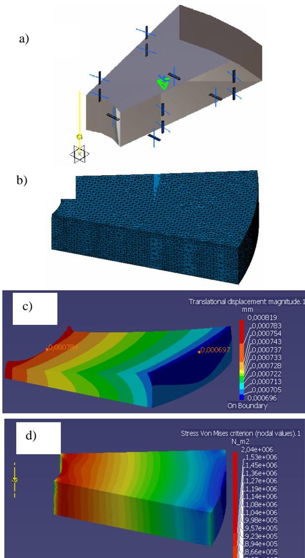
Fig.2. FEA modelling of a disc slice in rotation motion
