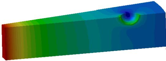
Fig. 4. Stress concentrator effect of a spherical indentation
