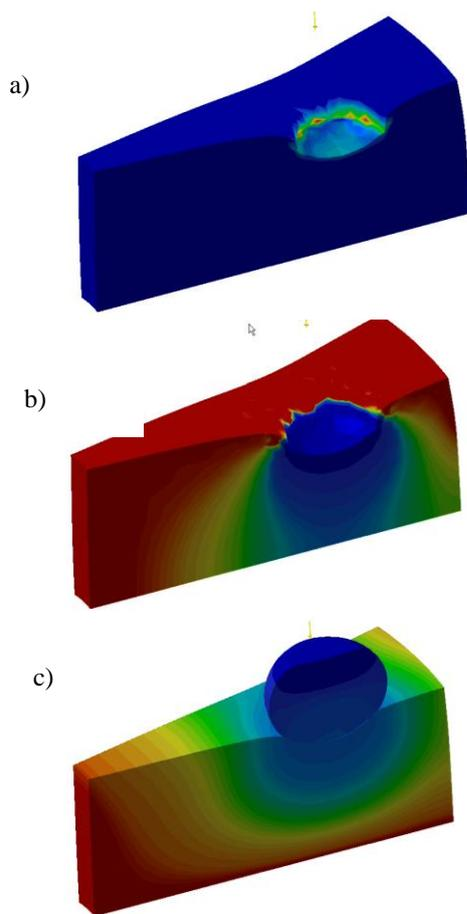
Fig. 6. Case of rotating disc: a) the equivalent von Mises stress; b) normal stress  $\sigma_z$ ; c) axial deformations
