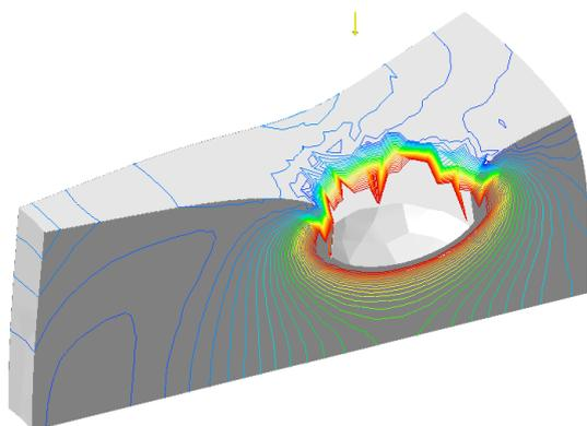
Fig. 7. The equivalent von Mises stresses, smaller than  $0.2\sigma_Y$
