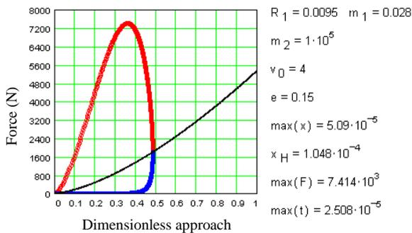
Fig. 5. Loading curves for elastic and dumped impact (loop)
