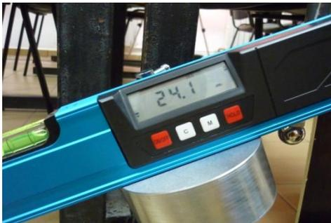
Fig. 7. Adjusting the tilt angle of the plane
