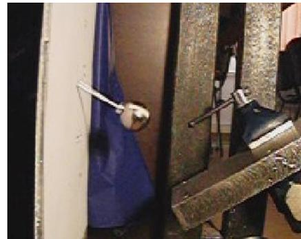
Fig. 4. The case when the metallic plate is in contact with the rod
