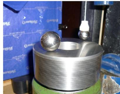
Fig. 8. Disc's deviation from horizontal plane test and contact point position identification
