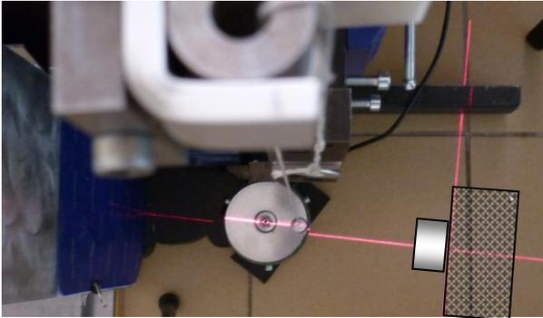
Fig. 2. Positioning of the video camera
