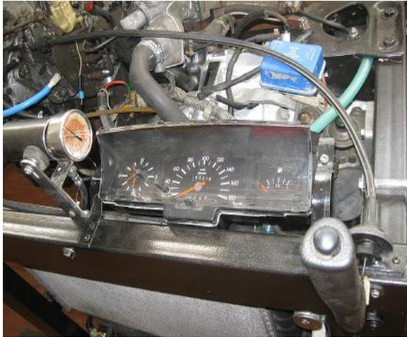
Fig. 2. The speedometer and the stand manometer
