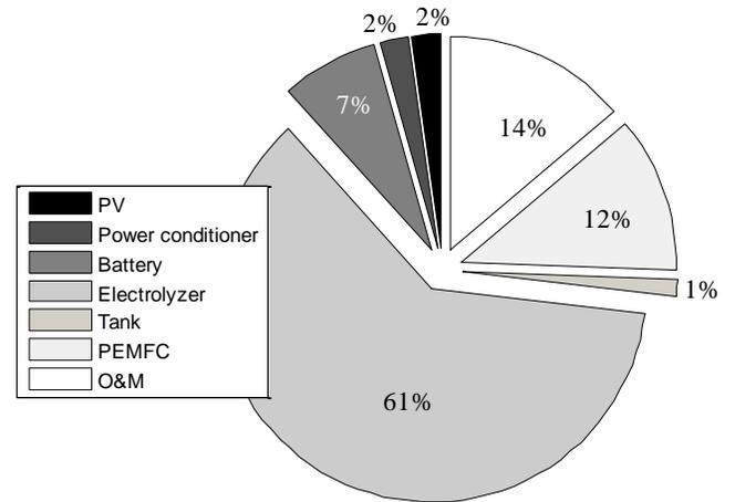
Fig. 5: The percentage cost of each component in the hybrid PV/PEMFC system over 30 years
