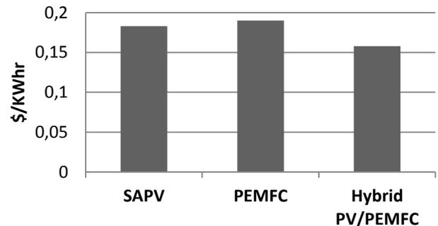
Fig. 6: The COE for three standalone alternative systems
