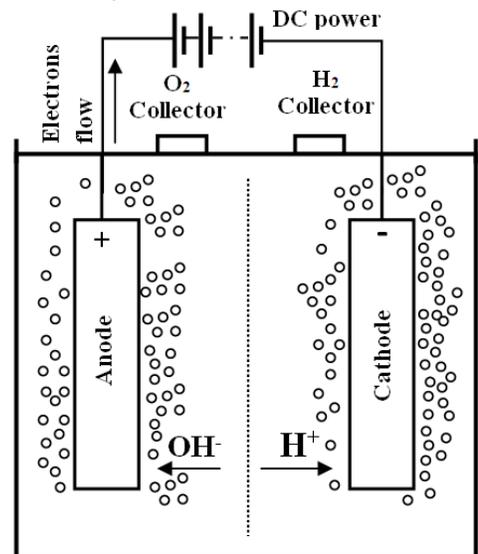
Fig. 1. Basic scheme of water electrolysis system
