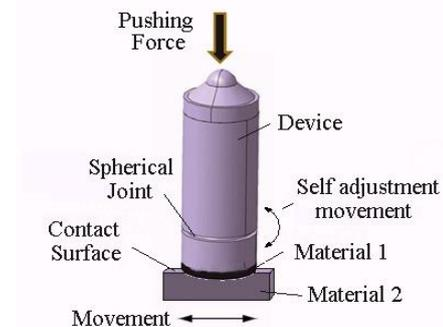
Fig. 2. The device with spherical joint, main parts and movements.
