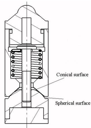
Fig. 5. Contact surfaces in spherical joint
