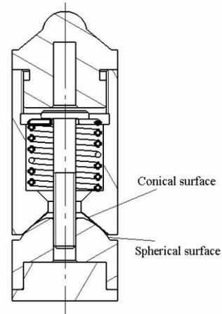
Fig. 5. Contact surfaces in spherical joint
