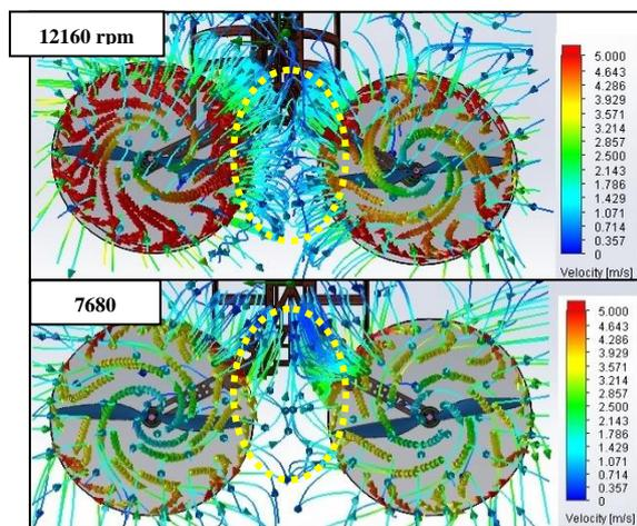
Fig. 8. Flow simulation around propeller
