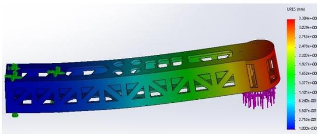
Fig. 4. Wing frame displacement analysis
