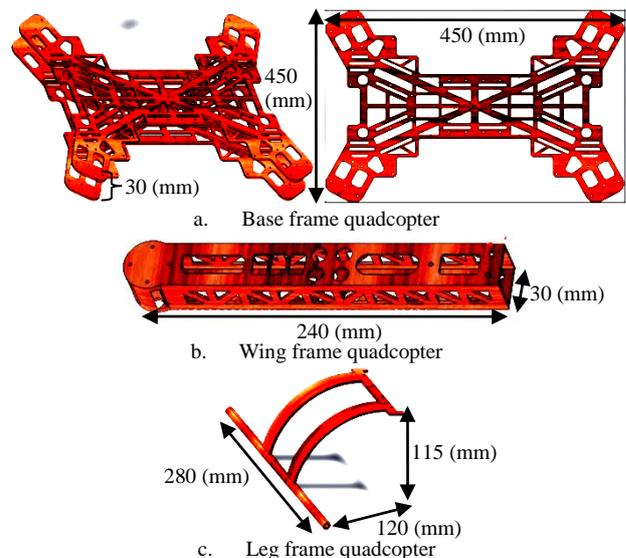
Fig. 1. The 3D CAD model for quadcopter
