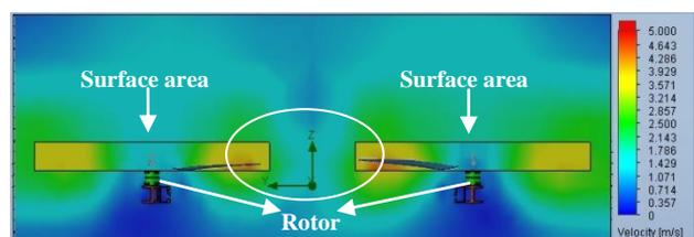
Fig. 7. Isosurface airflow between propellers with 7680 (rpm)
