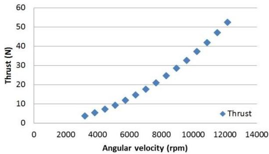
Fig. 3. Thrust for propeller 406x127 (mm)
