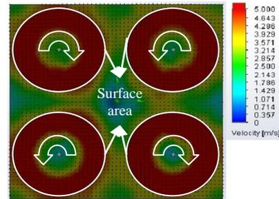
Fig. 5. Isosurface airflow around propeller
