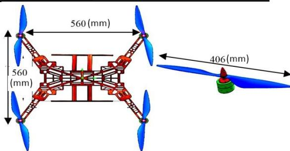
Fig. 2. Body frame quadcopter model
