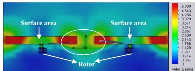
Fig. 6. Isosurface airflow between propellers with 12160 (rpm)
