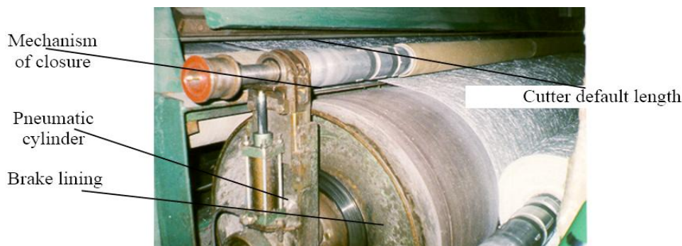
Fig. 11. The mechanism for fastening the prepared tubes for winding of MAT
