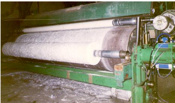
Fig. 12. The position of the prepared tubes for winding (upper position)
