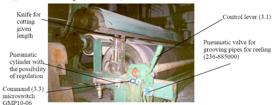
Fig. 10. Working (upper) position control levers
