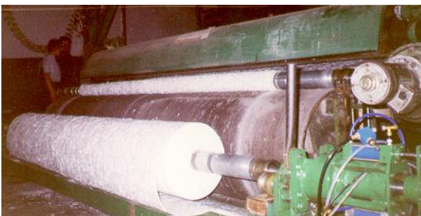
Fig. 13. The position of the new tubes for winding when it starts reeling in the upper tube
