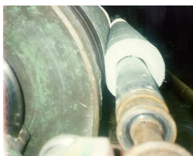
a) at the beginning of the winding b) at the end of the winding Fig. 2. Preview of the winding process with the first embedded solution of winding of MAT
