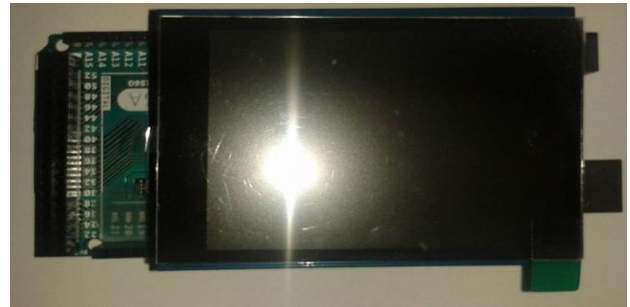
Fig. 8. TFT screen over Arduino board
