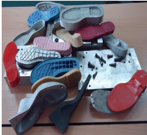
Fig. 9. Experimental injection mould with the interchangeable modular cavity and the soles manufactured using it. Solution 2.
