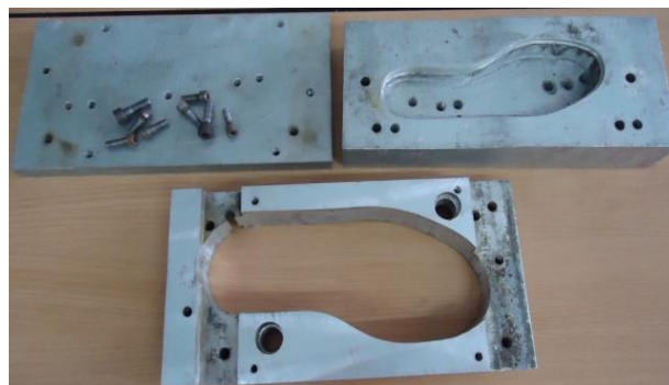
Fig. 7. Reusable parts of modular injection mould. Solution 2.
