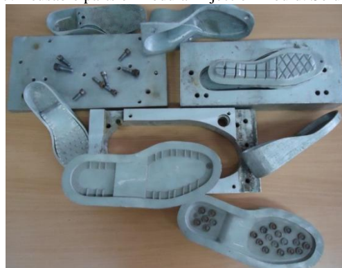
Fig. 8. Experimental injection moulds with an interchangeable modular cavity for prefabricated soles. Solution 2.
