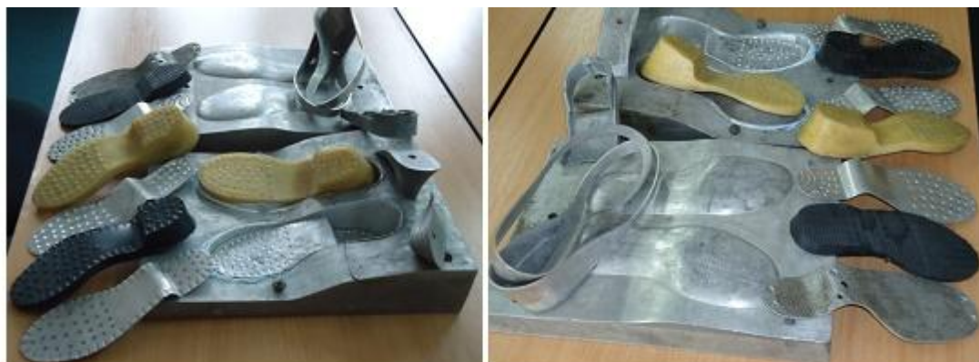
Fig. 4. Experimental injection mould with the interchangeable modular cavity and the soles manufactured using it. Solution 1a.
