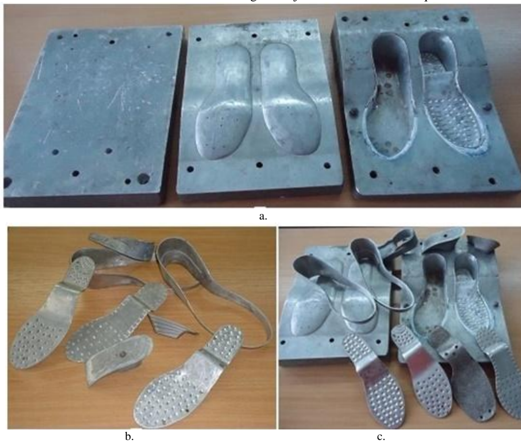
Fig. 3. Experimental injection moulds with an interchangeable modular cavity for prefabricated soles. Solution 1a.
