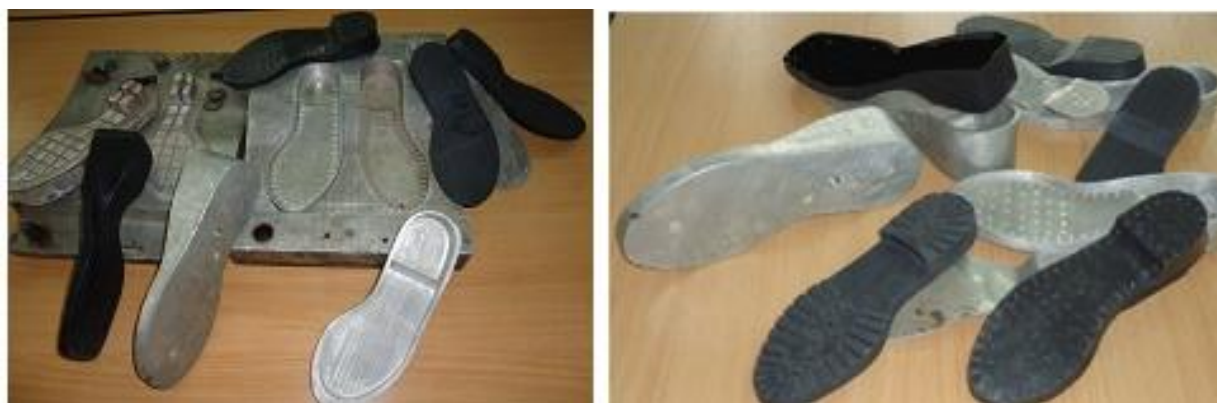
Fig. 6. Experimental injection mould with the interchangeable modular cavity and the soles manufactured using it. Solution 1b.
